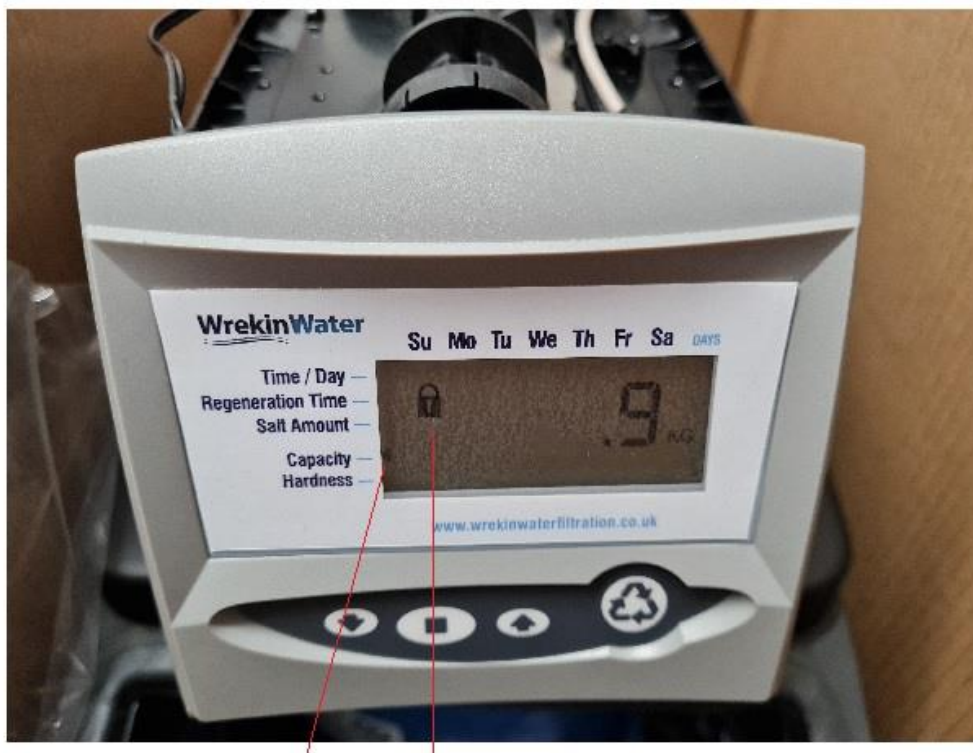
Capacity Setting - Factory set for model and locked to prevent accidental changing
